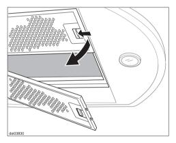
To remove the grease filters press the locking clips in towards the middle of the filter. Holding carefully, lower and remove the filter. Clean the filters
